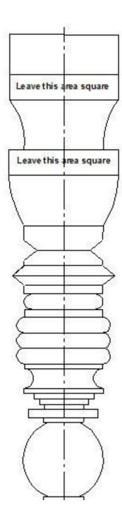
Bottom section of practice spindle turning shape. Put together with top section on previous page for full template.
