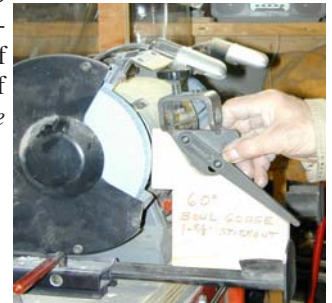
The side of the jig pocket is useful to measure stick-out
