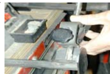
The side of the jig pocket is useful to measure stick-out
