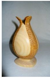
Tri-lobed vase turned on 3 separate axes
