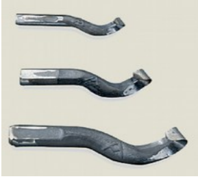
Andre Martel style hook tools. These are made as cutting tips that are inserted into shafts.
