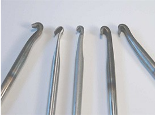
Standard shaped hook tools. These can be fairly easily made with a minimum of 'blacksmiths' tools or facilities.
