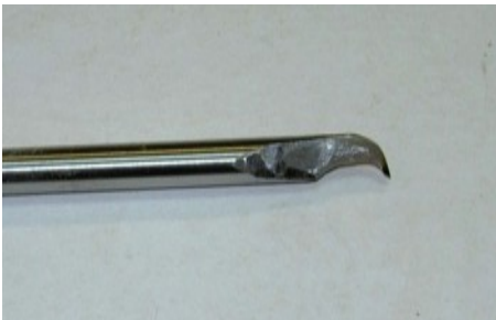
'Open' type of hook tool. This tool is harder to control when hollowing, more suitable for bowl work.
