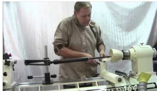
This system eliminates the capture 'slot' by using an articulated support system.
