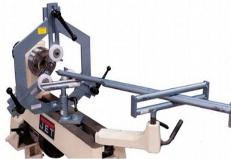
This hollowing system includes a steady-rest to hold fragile pieces while working deeper.
