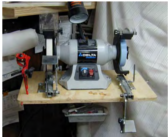
The TruGrind Sharpening system; RH sturdy rest is in “down” position, LH rest in “up” position. I can grind and sharpen all my woodturning tools here.
