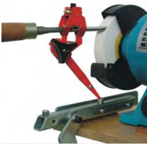
LH base, slide, tool clamp & sturdy rest in “down” position
